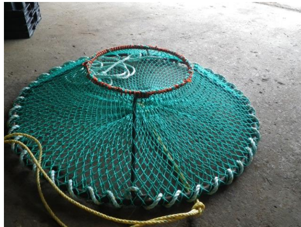
Figure 6 The trap used in Quebec (Canada) for whelk which has shown promise as a sea urchin trap.
